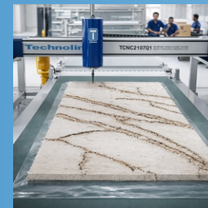
Cnc Quartz Slab Venas / Figuring Machine
